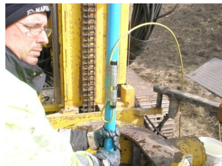
Figure 9. Transducer fastened upside-down to the standpipe.
