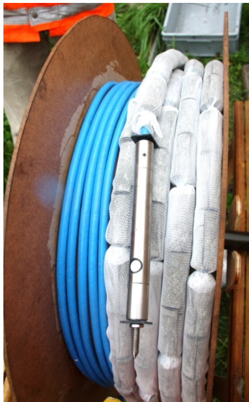
Figure 6: GeoBeads sensor string with integrated bentonite shells for hydraulic isolation between measurement depths.
