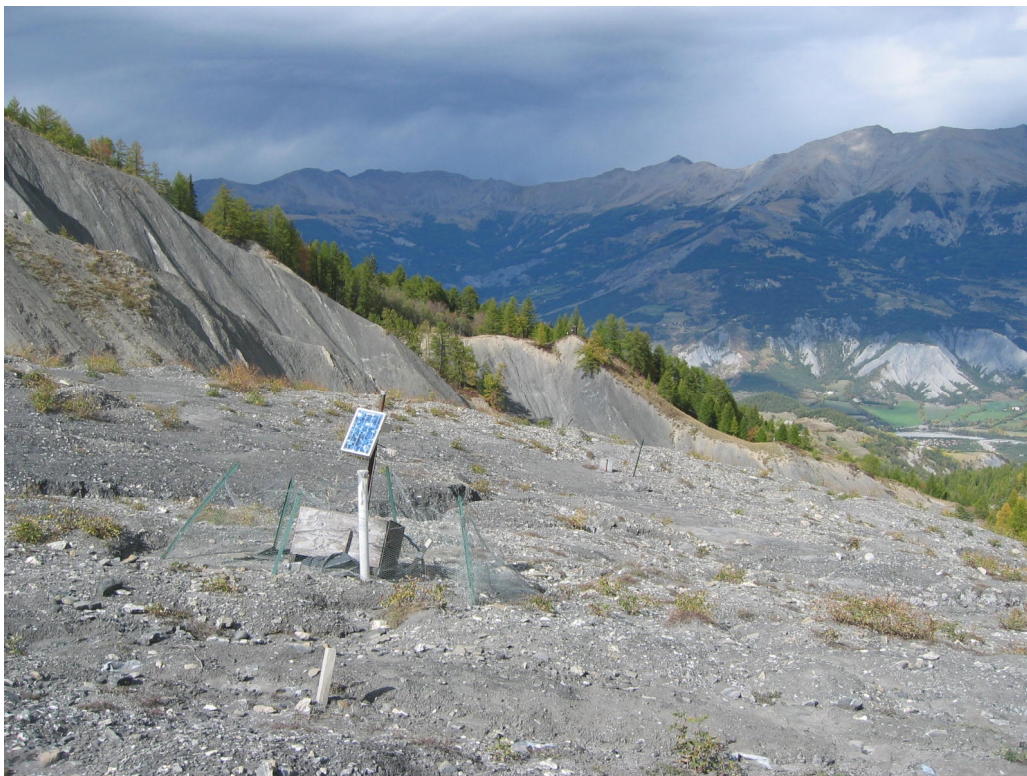
Figure 15: A GeoBeads measurement system on the Super-Sauze mudslide powered by a solar panel and set-up to travel along downhill with the mudslide.
