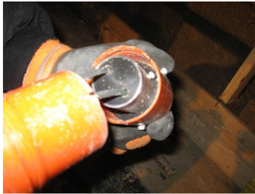
Figure 5. IPI casing end cap with pulley and cable attached.
