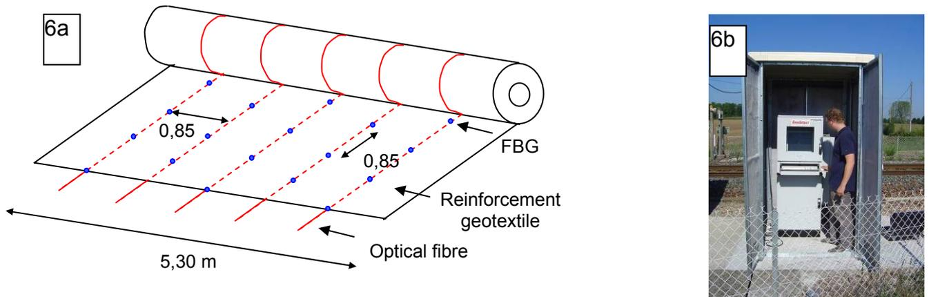
Figure 6. The fiber optics geotextile warning system installed below the railways line in the Arbois region. Distribution of the optical fibers and of the Fiber Bragg Gratings on the reinforcement geotextile (a) connected to the device for continuous measurement (b).
