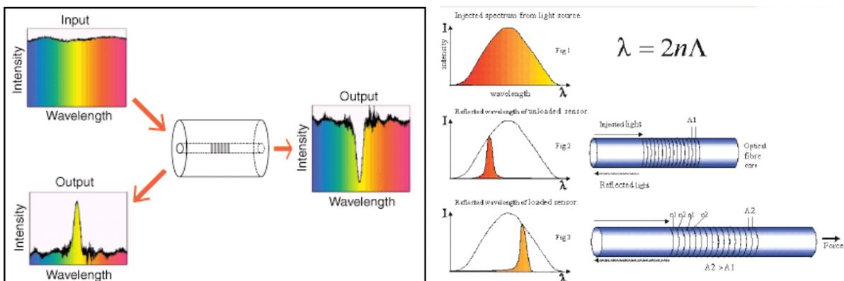
Figure 2. Principle of the Fiber Bragg Grating. (2a) : reflexion of a given wavelength (2a) and transmission of the remaining light spectrum. (2b) : the reflected wavelength is shifted as a linear function FBG strain.
