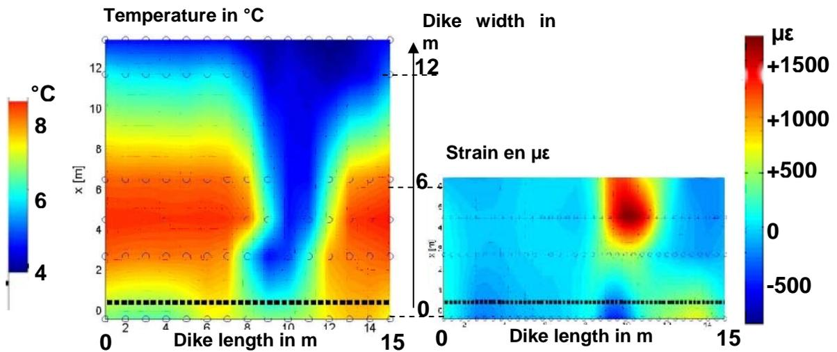
Figure 10. IJkdijk/Piping project - Detection of the piping channel below the dike (view from the top) by simultaneous measurement of temperature on the left and strain on the right.
