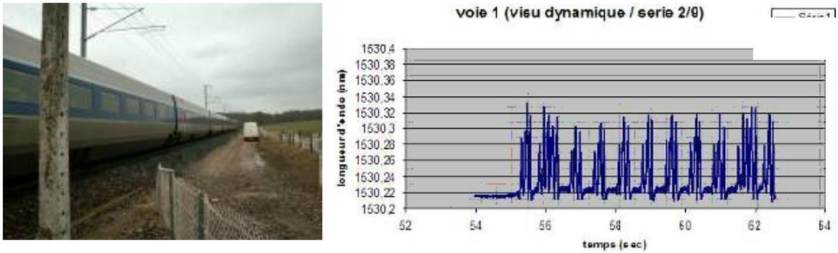
Figure 8. Railways in the Arbois area. Dynamic strain curve measured by the warning system during a train passes.
