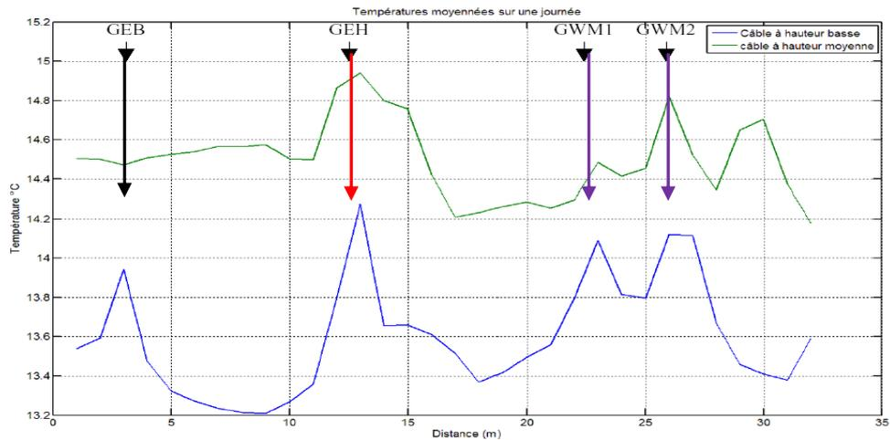
Figure 13. Detection of the artificial leaks (arrows) with the fiber optics geotextile enabled sensor for the sensor strip installed at the toe (blue curve) and at the middle (green curve) of the slope.
