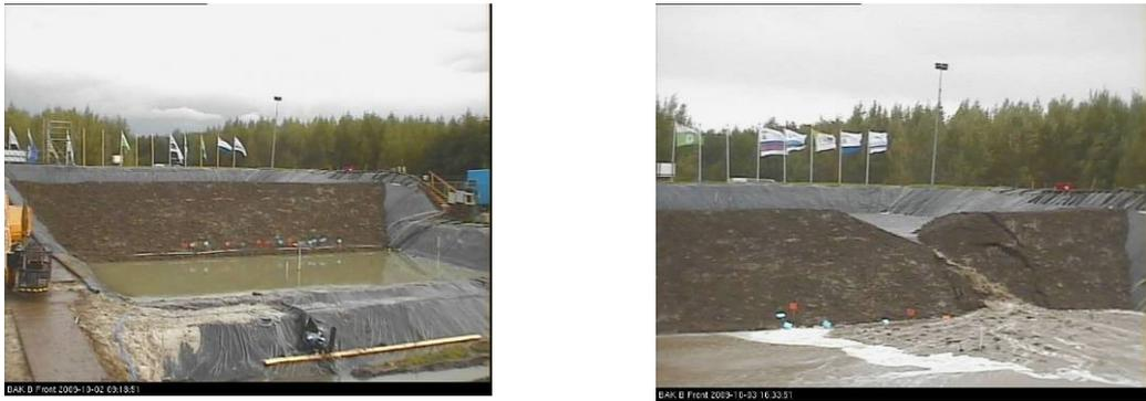
Figure 9. Project IJkdijk/Piping – An experimental dike before and after failure
