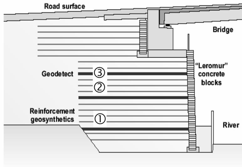
Figure 4. Cross section of the bridge abutment reinforced with geotextile in Saint-Saturnin and location of the 3 sensor strips.
