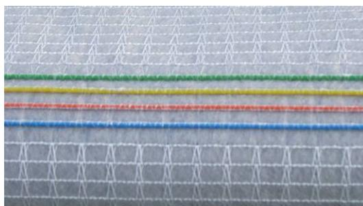
Figure 1. The textile composite sensor and the optical cables (colored).
